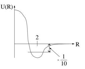
• The hypothetical H<sub>2</sub> molecules, interacting with each other through the van der Waals interaction, are assumed to have a single bound state of energy  $-1/10^2$  a.u. and the mean distance between the atoms is about  $\sim 10$ .
