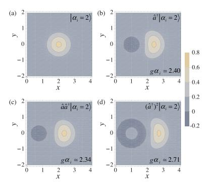
Fig. 2. Wigner functions of (a) a coherent state of amplitude  $\alpha_i = 2$  and the states after photonic operations, (b)  $\hat{a}^{\dagger}$ , (c)  $\hat{a}\hat{a}^{\dagger}$ , and (d)  $(\hat{a}^{\dagger})^2$ . The amplitudes of the amplified states,  $g\alpha_i$ , are noted for comparison.
