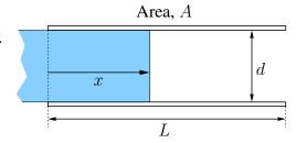
Now, as in the figure, let's try to insert a dielectric slab with  $\varepsilon_1$  into this capacitor. Let's assume that the whole set up is in the vacuum so that we have  $\varepsilon_0$  for the empty space  $(\varepsilon_1 > \varepsilon_0)$ .
