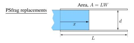
Now, as in the figure, let's try to insert a dielectric slab with  $\varepsilon_1$  into this capacitor. Let's assume that the whole set up is in the vacuum so that we have  $\varepsilon_0$  for the empty space ( $\varepsilon_1 > \varepsilon_0$ ).
